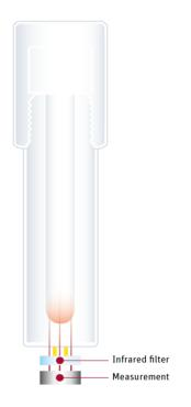
It is possible with this technology to detect the sample temperature in Teflon-vessels and their quartz inserts inside a microwave oven in a measurement range from 100 to 300 °C. The precision is relative high (+/-1 °C at 200 °C). Only through the precise knowledge of all sample temperatures inside the microwave oven the microwave power could be regulated in an optimal way.
