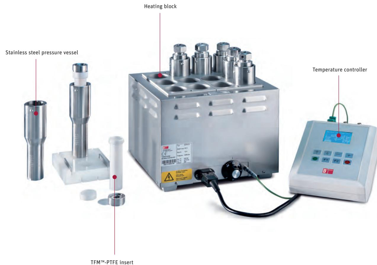
**Materials that are difficult to digest** or high sample weight represent a challenge for modern digestion instruments. Digestec by Berghof is distinguished by its high working pressure of up to 200 bar and offers the ideal solution for the most difficult samples. The decisive plus points are its simple filling and a digestion carried out under uniform heating that can be reproduced at any time.
