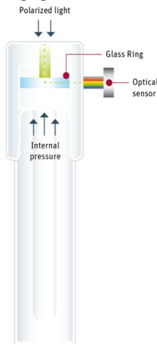
Figure 4: Contact-less measurement of pressure
