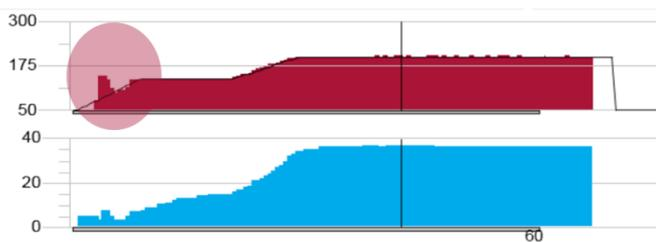
Figure 3: Temperature and pressure development during exothermic reaction
